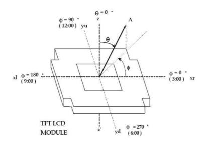
Viewing angle is the angle at which the contrast ratio is greater than 10.the angles are determined for the horizontal or x axis and the vertical or y axis with respect to the z axis which is normal to the LCD surface.
