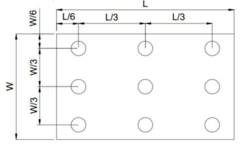
Lmax: The measured maximum luminance of all measurement position. Lmin: The measured minimum luminance of all measurement position.
