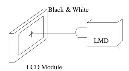
Fig. 6.3 The standard setup of CR measurement
