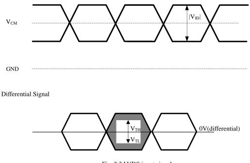
Fig. 3.3 LVDS input signal
