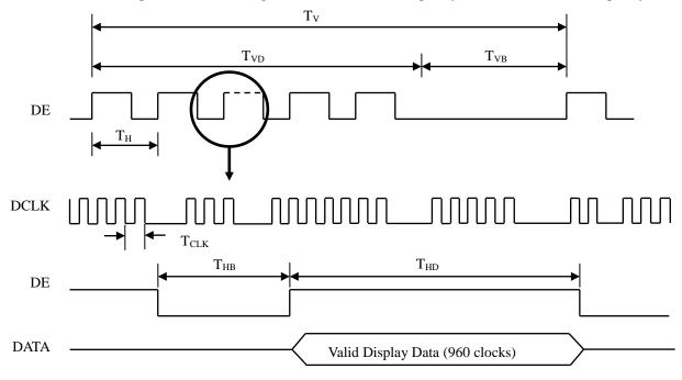
Fig. 5.1 Interface signal timing diagram
