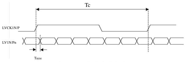
Fig.5.3 LVDS receiver interface timing diagram
