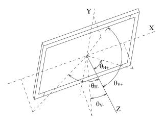
Fig. 6.6 Viewing angle coordination system
