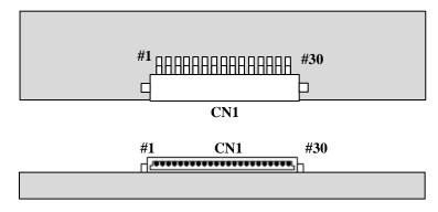
Fig. 4.1 LVDS connector direction sketch map
