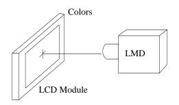
Fig. 6.5 The standard setup of color chromaticity measurement
