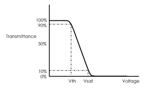
Figure 6. The definition of Vth & Vsat
