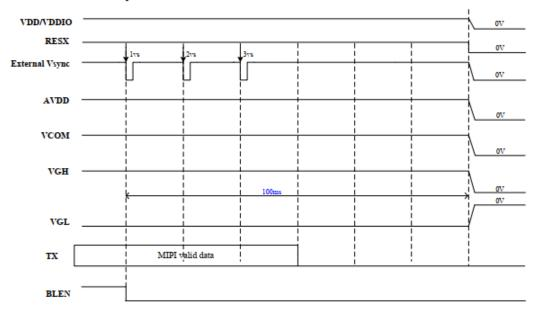
Figure : Power Off timing chart
