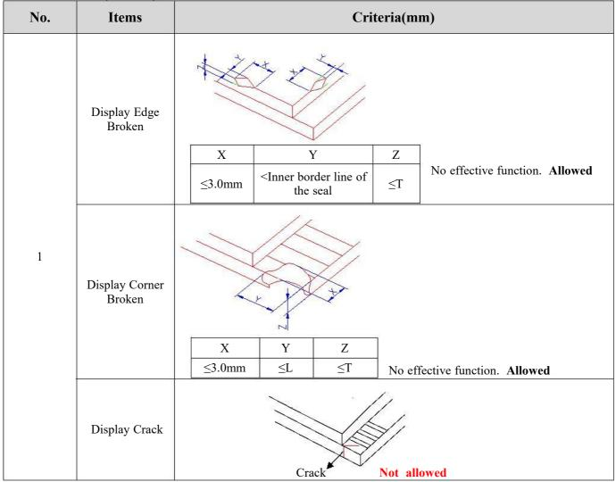
Notes: X=Length of defect, Y=Width of defect, Z=Height of defect, L=Length of ITO, T=Height of display.
