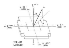
FIG.3. The definition of viewing angle视角定义
