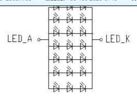
Figure 4.1 LED connection of backlight
