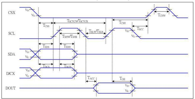
VDDI=1.65 to 3.3V, VDD=2.4 to 3.3V, AGND=DGND=0V, Ta=-30 to 70 ℃
