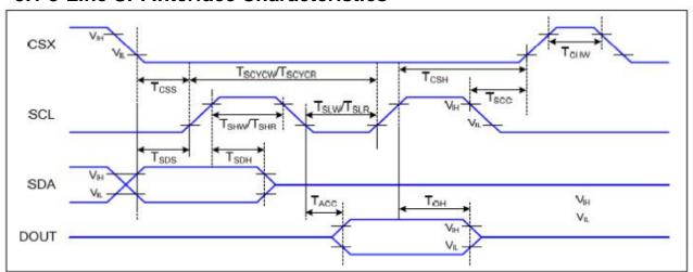
VDDI=1.65 to 3.3V, VDD=2.4 to 3.3V, AGND=DGND=0V, Ta=-30 to 70 ℃
