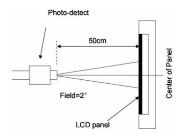
Figure 4 Optical test equipment.
