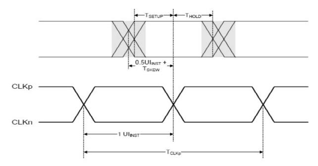
Figure 7-1 DSI HS UI timing definition
