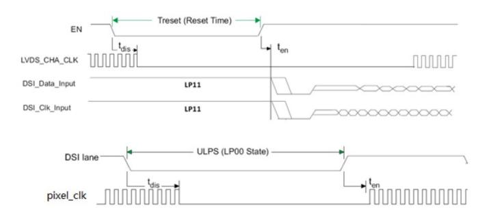
Figure 7-4 Power on and RESET and ULPS timing
