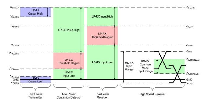
Figure 7-2 DSI HS/LP signaling and Contention Voltage
