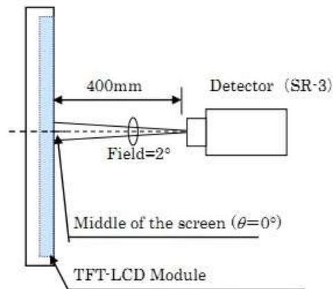
[Note 9-1] Fig.9-1 Measurement of Viewing angle range and Response time. (Viewing angle range: EZ-CONTRAST, Response time: Photodiode)
