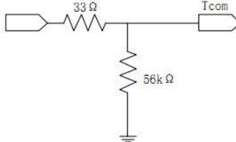
Fig.4-1-2 Equivalent circuit (Pin No.23)
