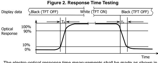
The electro-optical response time measurements shall be made as shown in FIGURE 3 by switching the "data" input signal ON and OFF. The times needed for the luminance to change from 10% to 90% is Tr and 90% to 10% is Td.
